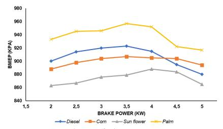
Figure 2. Break mean effective pressure vs brake power
