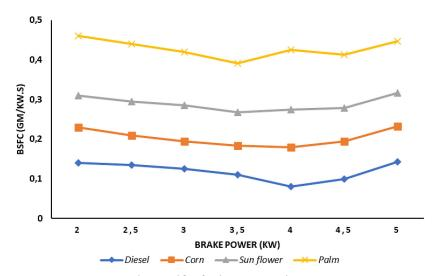
Figure 4. Break-specific fuel consumption vs brake power
