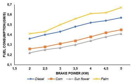
Figure 3. Fuel consumption vs brake power
