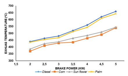
Figure 5. Exhaust gas temperature vs brake power
