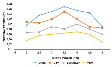
Figure 6. Thermal efficiency vs brake power
